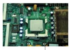
Socket lever in the locked position
